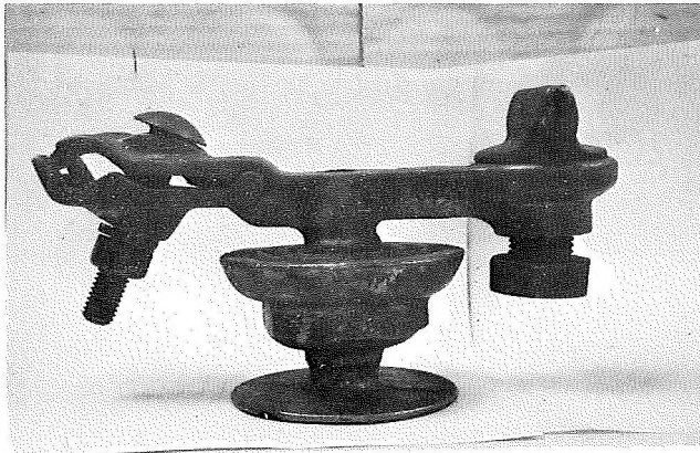
Trolley Feed Wire (Fig. 8) Insulator from an abandoned mine. embossed OHIO BRASS, and DUKANE BULLDOG
