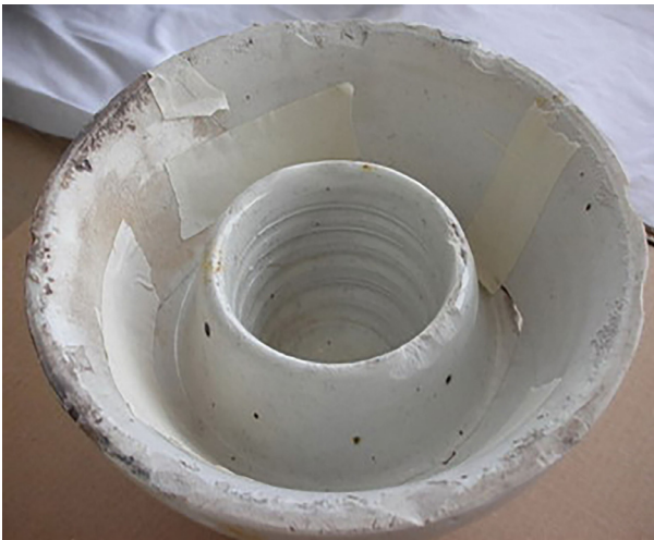
NOTICE THE INNER RIDGES OF THE M-2201 TO HOLD SULPHUR OR CEMENT THE THE ADDED INNER SKIRT
