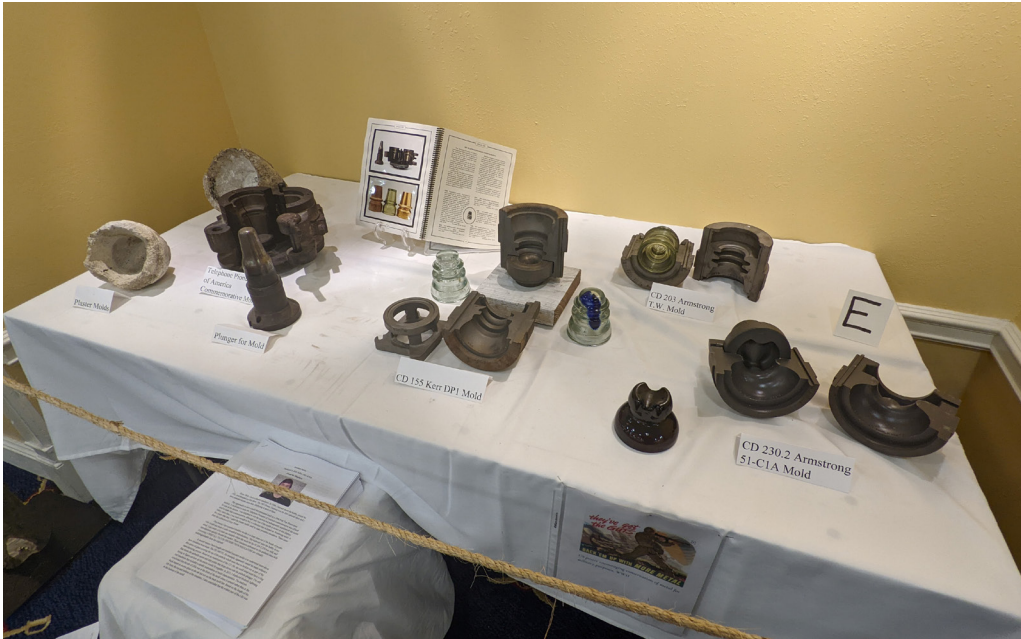
RICK SOLLER'S DISPLAY OF INSULATOR MOLDS, INCLUDING MOLDS FROM THE ARMSTRONG 203 AND 230.2, THE KERR CD 155, AND THE TELEPHONE PIONEERS COMMEMORATIVE.
