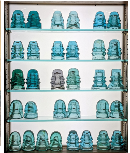
THREADED AND THREADLESS COUNTERPARTS FROM THE SAME MOLDS. ALL ARE PERFECT MATCHES EXCEPT WHICH PLUNGER WAS USED TO FORM THE INTERIOR.
