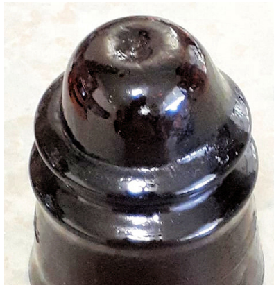
ABOVE: AN AMBER 423 WITH A LARGE SLUMP IN THE DOME GLASS
