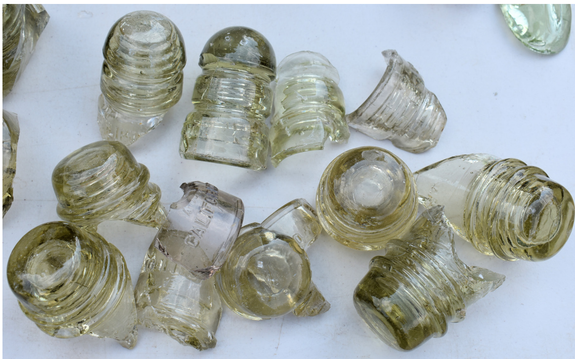
FIGURE 30 - CLEANED BROKEN SPECIMENS OF YELLOW CD 114 KEGS AND CD 121 TOLLS
