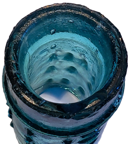
FIGURE 15 - THE INSIDE "DIMPLES" OF A CD 723
