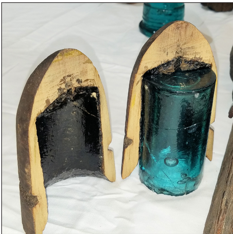
FIGURE 7 - A CD 723.3 INSIDE A SPLIT COVER, SHOWING HOW THESE UNIQUE INSULATORS FIT WITHIN THEIR PROTECTIVE OUTER WOODEN SHELL
