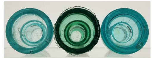
BASE COMPARISONS: LEFT (16 B'WAY BLOT OUT). CENTER: CLASSIC OR REGULAR 735 TILLOTSON. RIGHT: (NON BLOT-OUT) NOTE ITS VERY THICK BASE. ALSO, BOTH NEW YORKER INSULATORS (RIGHT AND LEFT) HAVE ROUNDED BASES, WHEREAS THE CLASSIC 735 TILLOTSONS HAVE FLATTENED BASES
