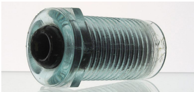
THE FLOOR TUBE "TURDUCKEN" – DWAYNE ANTHONY SHARED THIS UNIQUE FLOOR TUBE FIND WITH ME; APPARENTLY ONE TUBE WASN'T ENOUGH, SO SOME CREATIVE ELECTRICIAN WRAPPED RUBBER AROUND A PORCELAIN FLOOR TUBE AND SHOVED IT INSIDE A GLASS FLOOR TUBE!
