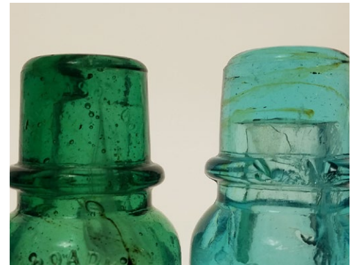
THE NON-BLOT OUT VERSION APPEARS TO BE A DIFFERENT MOLD. THE WIRE CHANNEL IS SLIGHTLY WIDER AND THE SHOULDER SLOPE DROPS A LITTLE MORE QUICKLY THAN A NORMAL TILLOTSON
