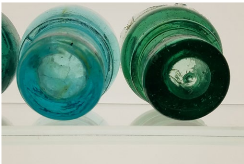
THE POINT AT THE TIP OF THE DOME, WHICH IS TYPICAL OF THE TOP AND CENTER OF THE INNER DOMES OF CLASSIC 735 TILLOTSONS, SEEMS TO BE ABSENT IN THE NEW YORKERS
