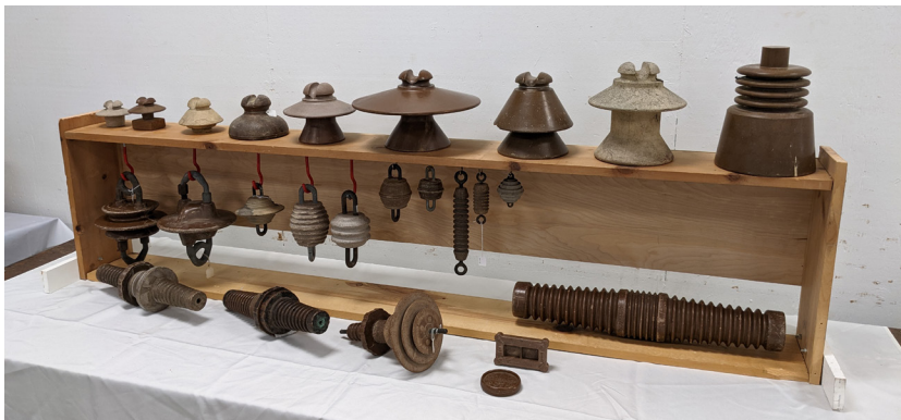
RICK SOLLER'S OTHER DISPLAY - A DISPLAY OF MANY RARELY-SEEN VARIETIES OF "ELECTROSE" COMPOSITE INSULATORS
