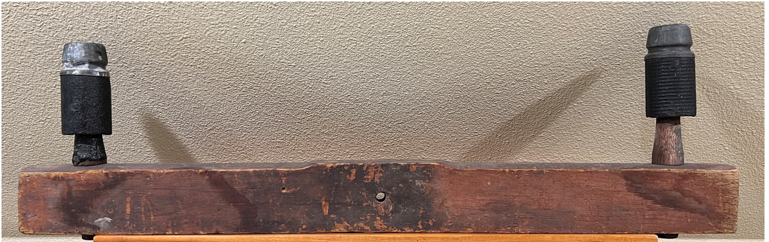
FIGURE 15 - ORIGINAL CROSSARM WITH TWO POND INSULATORS
