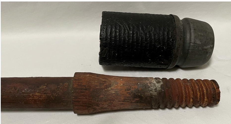
FIGURE 13 - AN UNEMBOSSED THREADED POND (2-1/4" X 4-1/2") AND A PIN
