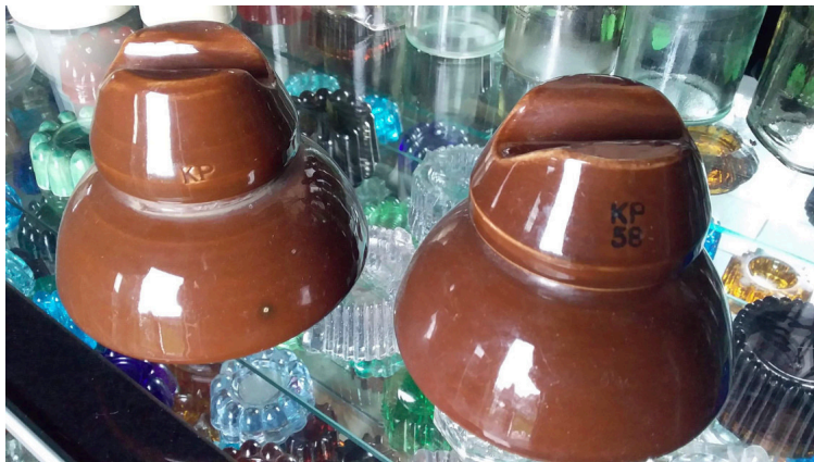
5,000 VOLT PIN TYPES WITH INCUSE & UNDER GLAZE MARKINGS
