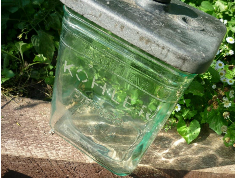
← 76.13 is a Philco battery jar with the brand name KOHLER embossed on the front. Full embossing is Water Level / KOHLER / Philco / Made In U.S.A. Dimensions are approximately 4" x 7" x 12" tall.
