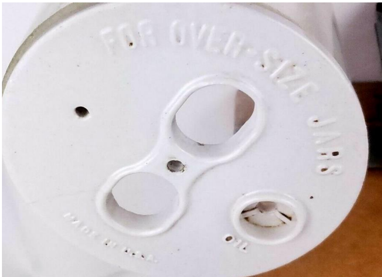
← 36.18 shows one of the original lids from the Carbonaire jars in 8. The lids are white porcelain and embossed: (arc) FOR OVER-SIZE JARS / MADE IN U.S.A. Like we've see on other lids these, too, have separate a separate hole for adding battery oil. It is so marked.
