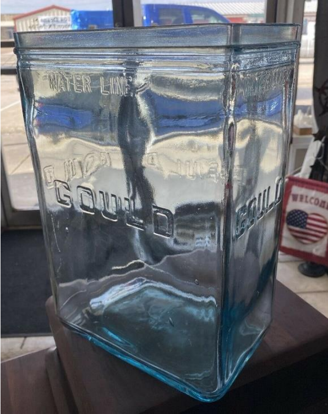
← 51.3 is a blue battery jar also with the Gould name. It is embossed WATER LINE / GOULD on all four sides. Its dimensions are 6" x 9" x 13" tall. Courtesy of Tommy Bolack
