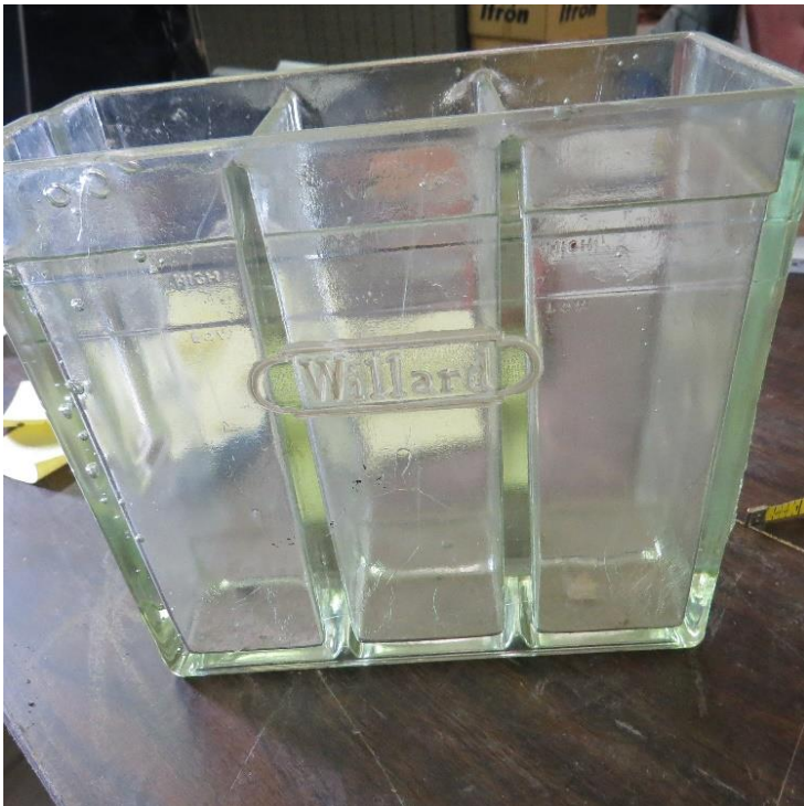
← 10.4 This Willard uranium glass jar has dimensiona of 8.75" x 4" x 7.75" tall. Each cell is 2.5" x 3.25" x .,75" tall. It also would have provided 6 volts. Courtesy of Tommy Bolack
