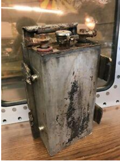
← 36.13 shows an Edison Alkaline Battery from the early 1900s.
