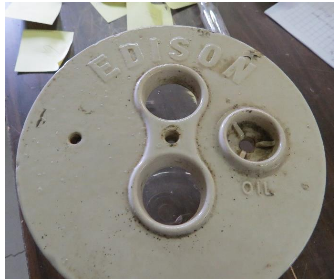
← 106.119 and 106.120 ↑ show an unembossed jar in light lavender with an EDISON lid. The jar is 6.75" diameter x 8.25" tall; 8.5" with the lid. Courtesy of Tommy Bolack
