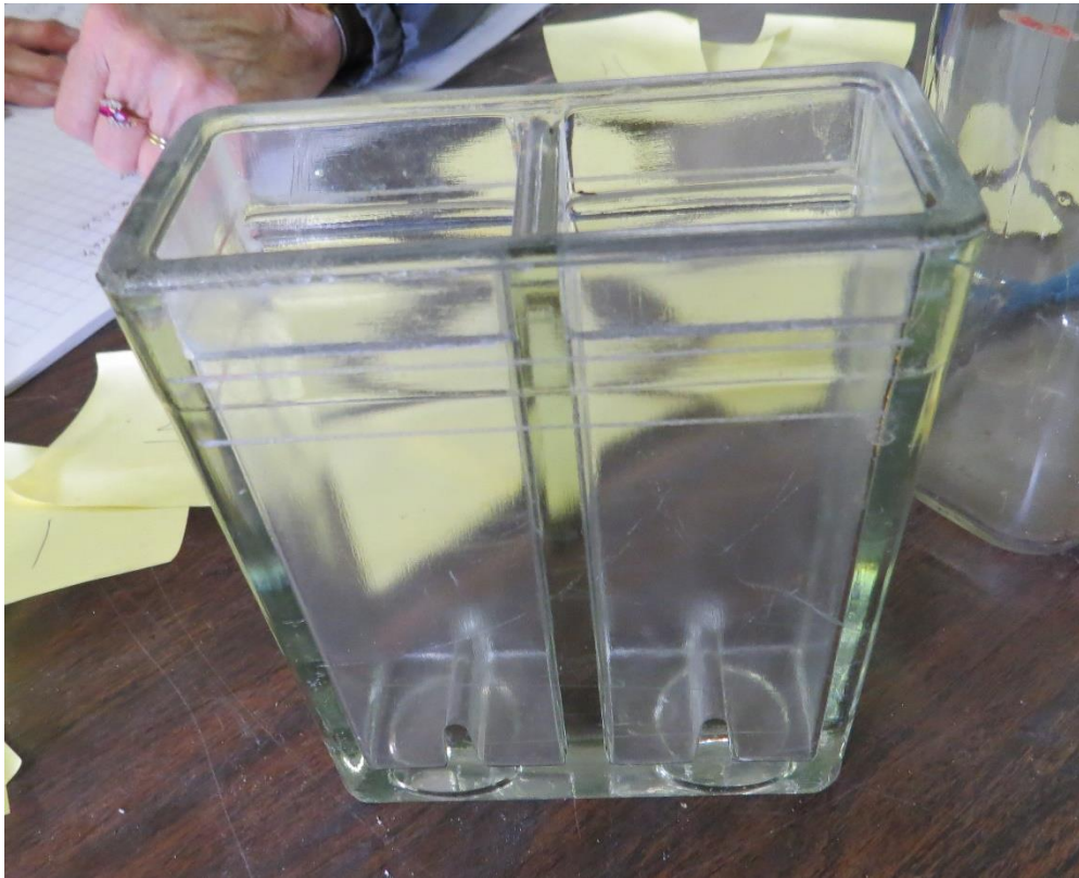
← 106.150 is an unembossed double cell with base dimensions of 1.75" x 2.375" x 5.75" tall Courtesy of Tommy Bolack
