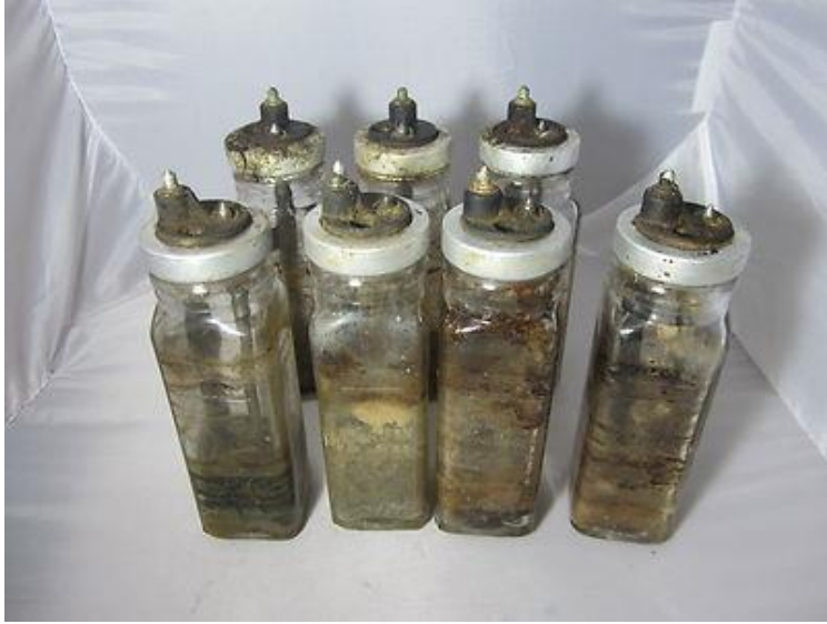
← 13.09 shows radio rectifier cells from Philco.
