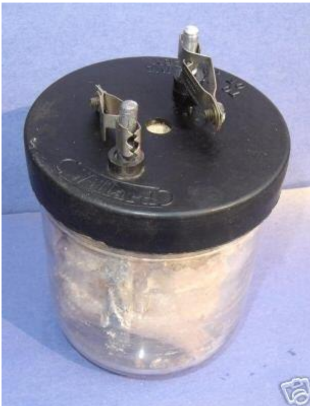
← 13.08 is a rectifier cell from Willard.
