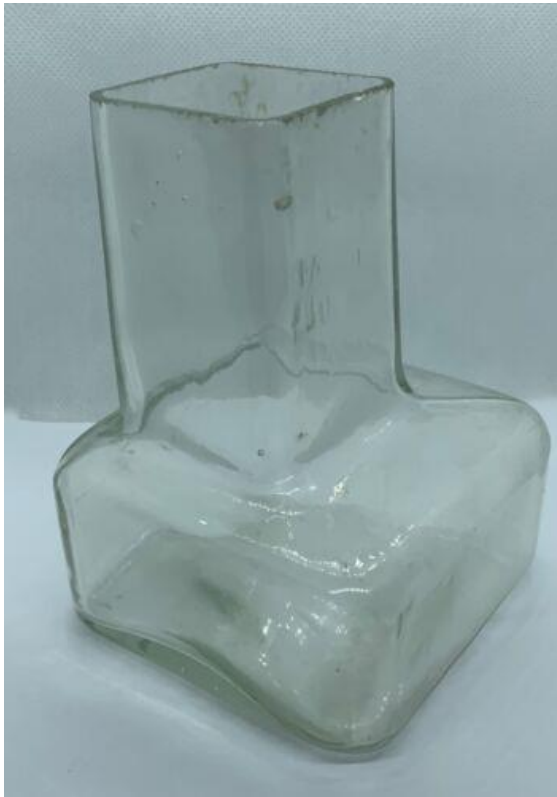
14.1 The Grenet or Poggendorf batteries such as this from Whitall Tatum were used to power Edison phonographs.
