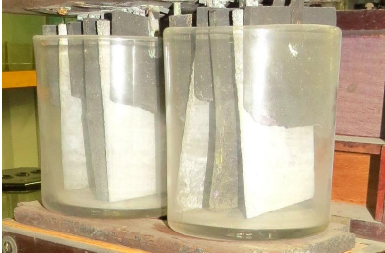
← 106.108 shows two unembossed battery jars. They are small, with dimensions of only 3.5” diameter x 5” tall. Courtesy of Tommy Bolack.
