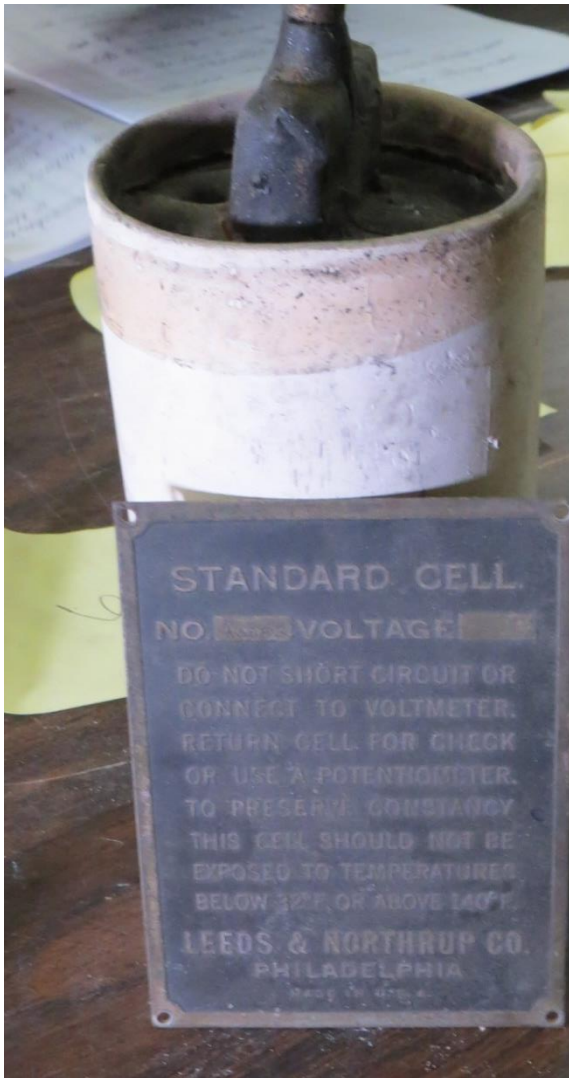
← 60.1 is a STANDARD CELL from Leeds & Northrup . The dimensions are 3" diameter x 5.5" tall. Courtesy of Tommy Bolack
