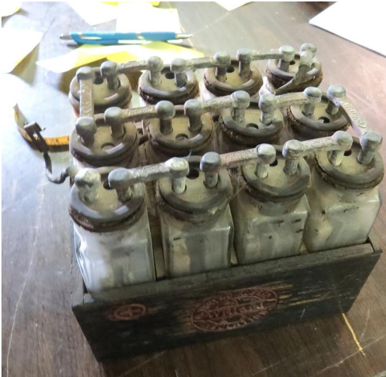
← 102.10 is a WILLARD radio battery. it has 12 cells in an array. Each cell is 1.5" x 5" tall. The box is labeled (Arc) THREAD RUBBER / WILLARD / (arc) INSULATION . Another side is labeled Part No 2833. Courtesy of Tommy Bolack.
