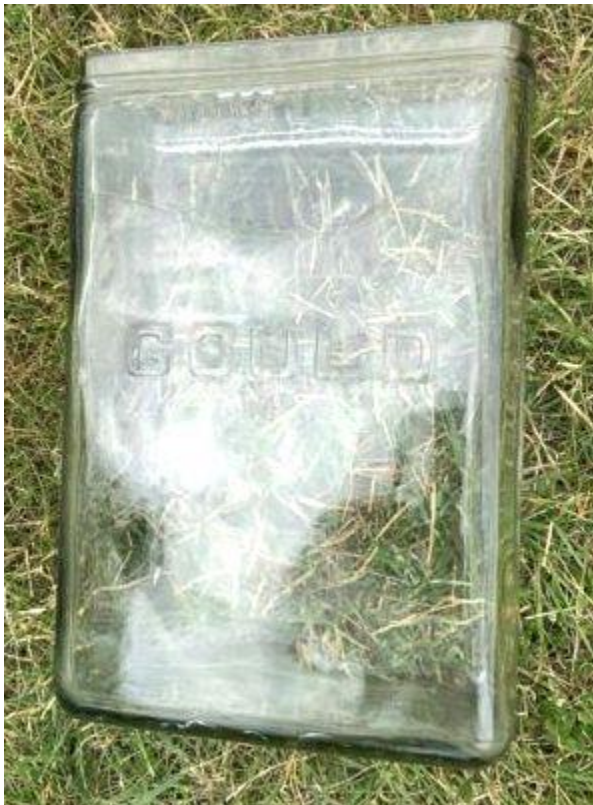
← 51.4 is a clear glass GOULD battery jar. It has dimensions of 3.75" x 8" x 13" tall. It is embossed WATER LINE / GOULD on two sides.
