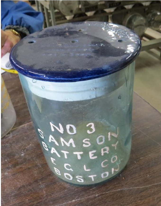
← 38.10 and 38.11 show a NO 3 / SAMSON BATTERY / EGL CO. / BOSTON battery jar with a (arc) GLADSTONE LALANDE BATTERY lid. It has three patent dates and is the same lid as 40 - 5. Courtesy of Tommy Bolack
