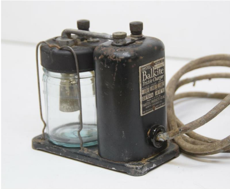
← 13.07 is trickle charger for radios, from Fansteel. Courtesy of Walt Baumgardt.
