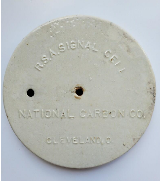
12.4 is an R.S.A. Signal Cell lid from the National Carbon Co. of Cleveland, Ohio.
