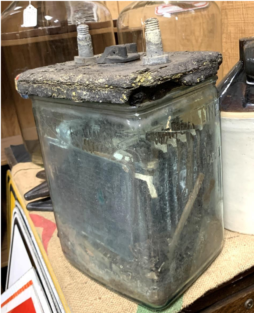
32.32↑ is embossed WATER LINE / DELCO LIGHT / EXIDE on all four sides. The dimensions are 6" x 7" x 11" tall.
