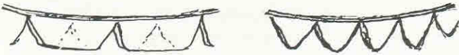
(Figure 5.) The Star wedge drip point (left) is a combination of two standard drip points bridged with a slug of glass. (left) The drip points on the right are the standard style of molding.
