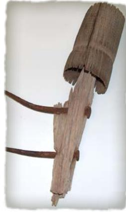
The vulcanized rubber insulator insert is 3 1/2 inches tall, 1 1/8 inches in diameter at the top, and 1 5/8 inches in diameter at the bottom. The sides begin to flare out in a gentle curve 2 5/8 inches down from the top. It would be great to know how many of these pieces exist.
