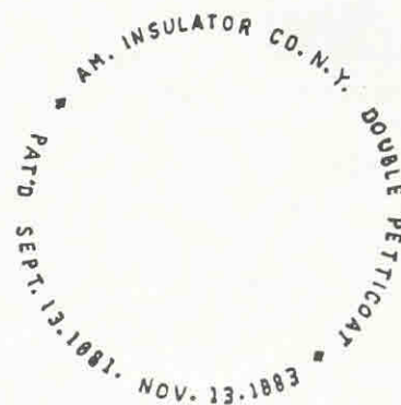
(Figure 2.) Smaller, fine lettering which appears on American Insulator Co. CD 160.7 insulators.
