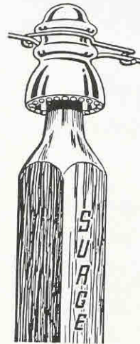
SURGE Fencer Post
