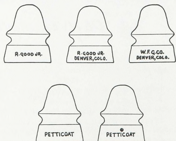
(Figure 3.) CD 162 signals illustrating the progression of embossing changes produced by Robert Good, Jr.
