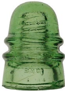
Figure 1. Measure the height and width of the insulator and create a grid (1/8" for large, 1/16" for small) rectangle matching those dimensions. Add a vertical center line and center it on the rectangle.
