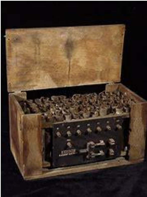
← 36.14 shows an early Edison Battery Tube Radio. Note the array of batteries.
