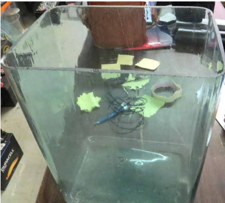
← 106.106 is another unembossed battery jar. It has a ground lip, with dimensions of 8.5" x 12.75" x 17" tall. Courtesy of Tommy Bolack.
