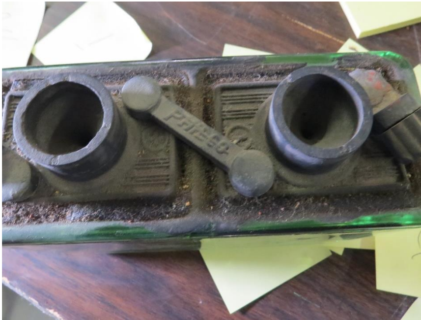
← 10.6 This two cell PHILCO jar is also in uranium glass. With dimensions of 7" x 2.75" x 5.75" tall, (each cell 3" x 2" x .25" tall), it could have been a jar for an electric vehicle. I suspect, however that it is actually a radio battery. Courtesy of Tommy Bolack.
