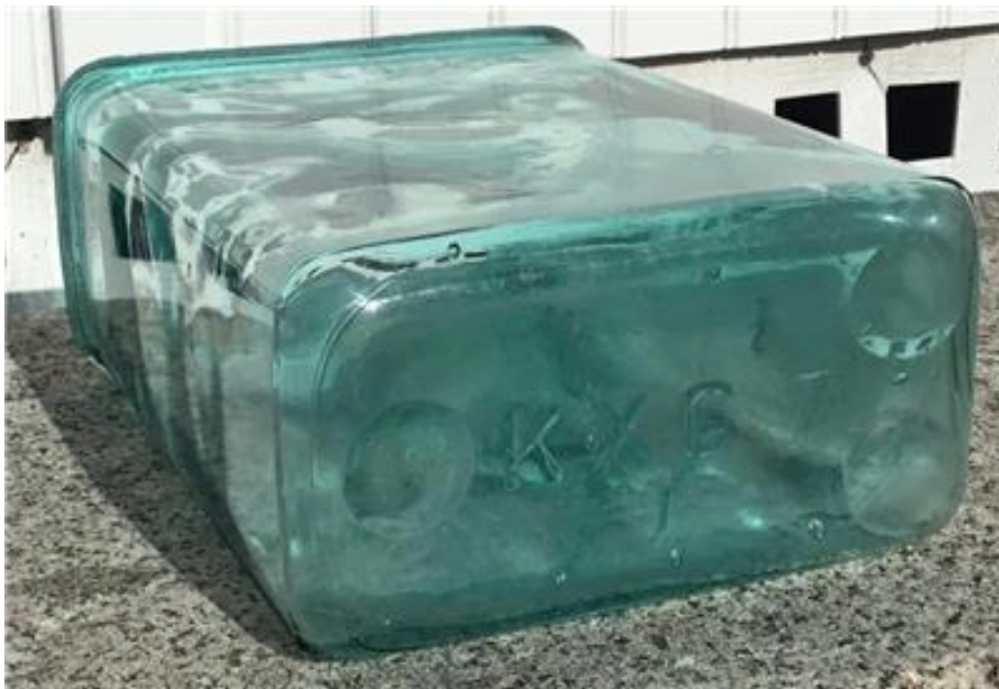
← 32.15 is a Delco Light Exide battery jar with dimensions of 3.5" x 7.25" x 10'25" tall. It is embossed KXG – 7 on the bottom. It is embossed on 4 sides: WATER LINE / DELCO LIGHT / EXIDE . On 2 sides it is embossed MADE IN U.S.A. near the bottom.
