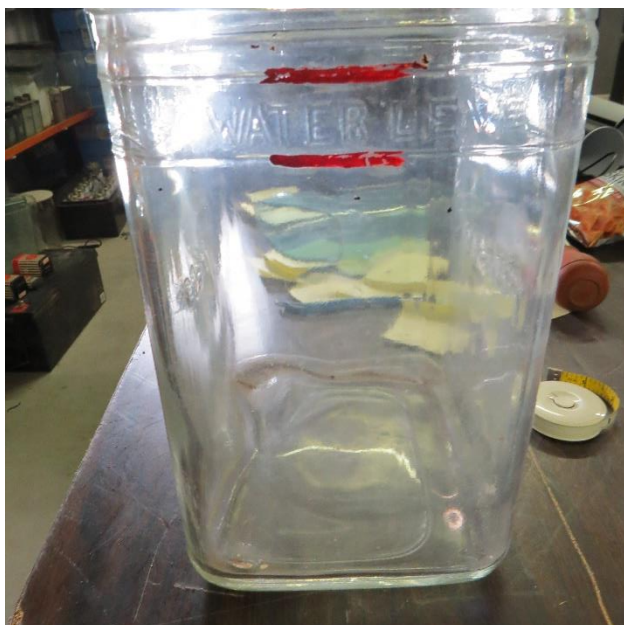
←47.14 is embossed High and Low Water Lines on 4 sides and PHILCO two opposing sides with G - 12 on the bottom. The dimensions are 6" x 7.75" x 10.25" tall. Courtesy of Tommy Bolack
