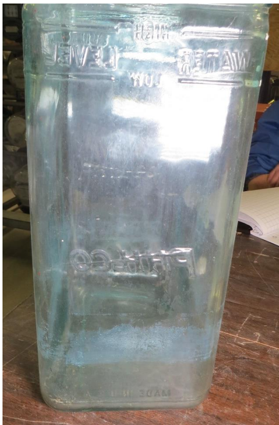
←47.12 and 47.13↑ show a PHILCO battery jar. It is embossed HIGH and LOW WATER LINE / PHILCO on 4 sides, with G -17 on the bottom. The dimensions are 6.25" x 9.25" x 14" tall. Courtesy of Tommy Bolack
