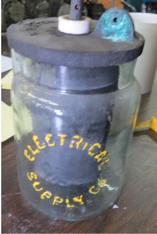
← 106.154 is marked (arc) ELECTRICAL / (arc) SUPPLY CO. with dimensions of 4.375 x 5.75" tall. The lid, 140 and electrode, 106.155, is embossed V.B.E. Co / PHILA PA. Courtesy of Tommy Bolack
