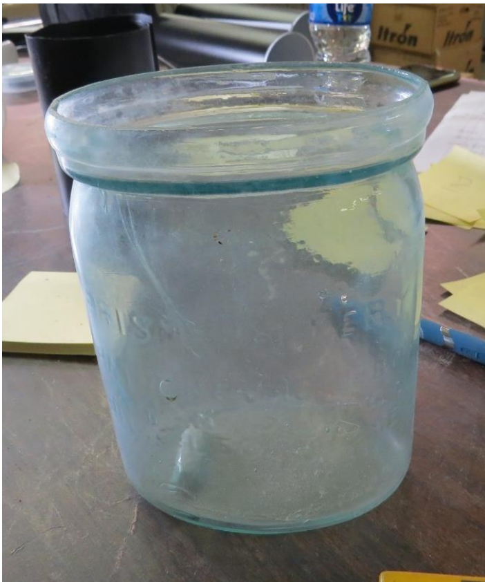
← 24.1 is embossed PRISM BATTERY / CALIFORNIA / ELECTRICAL WORKS . The jar is oval with dimensions of 3.25" x 4.4" x 6" tall. Courtesy of Tommy Bolack.
