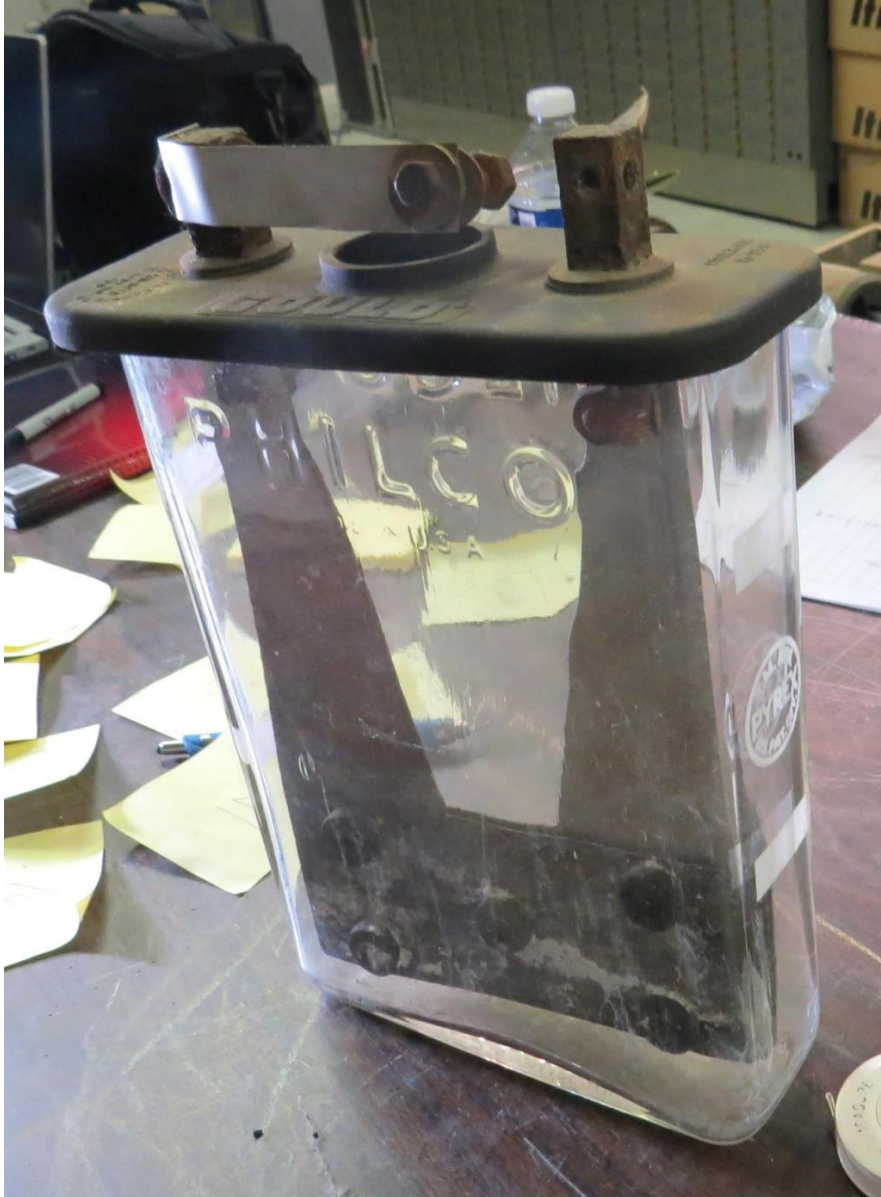
76.18↑ is a Philco jar, manufactured by Corning with a Gould Lid. The jar is embossed PHILCO / U.S.A. on opposing sides. The dimensions are 2.5" x 6.75" x 9" tall; 9.5" with the lad. It is fair to assume the lid is not original. Courtesy of Tommy Bolack
