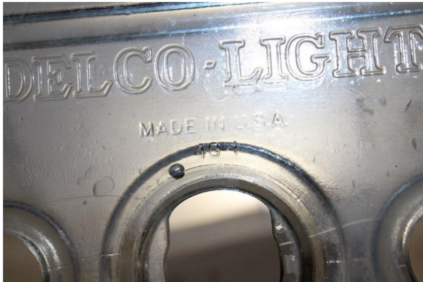
← 32.14 shows a DELCO LIGHT battery jar lid. Its dimensions are 8" x 7", indicating it fit a jar with top dimensions of 7" x 6". It is embossed DELCO – LIGHT / MADE IN U.S.A. , with numbers 46 – 1 and 21959 .
