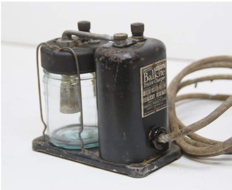
← 13.7 is trickle charger for radios, from Fansteel. Courtesy of Walt Baumgardt.
