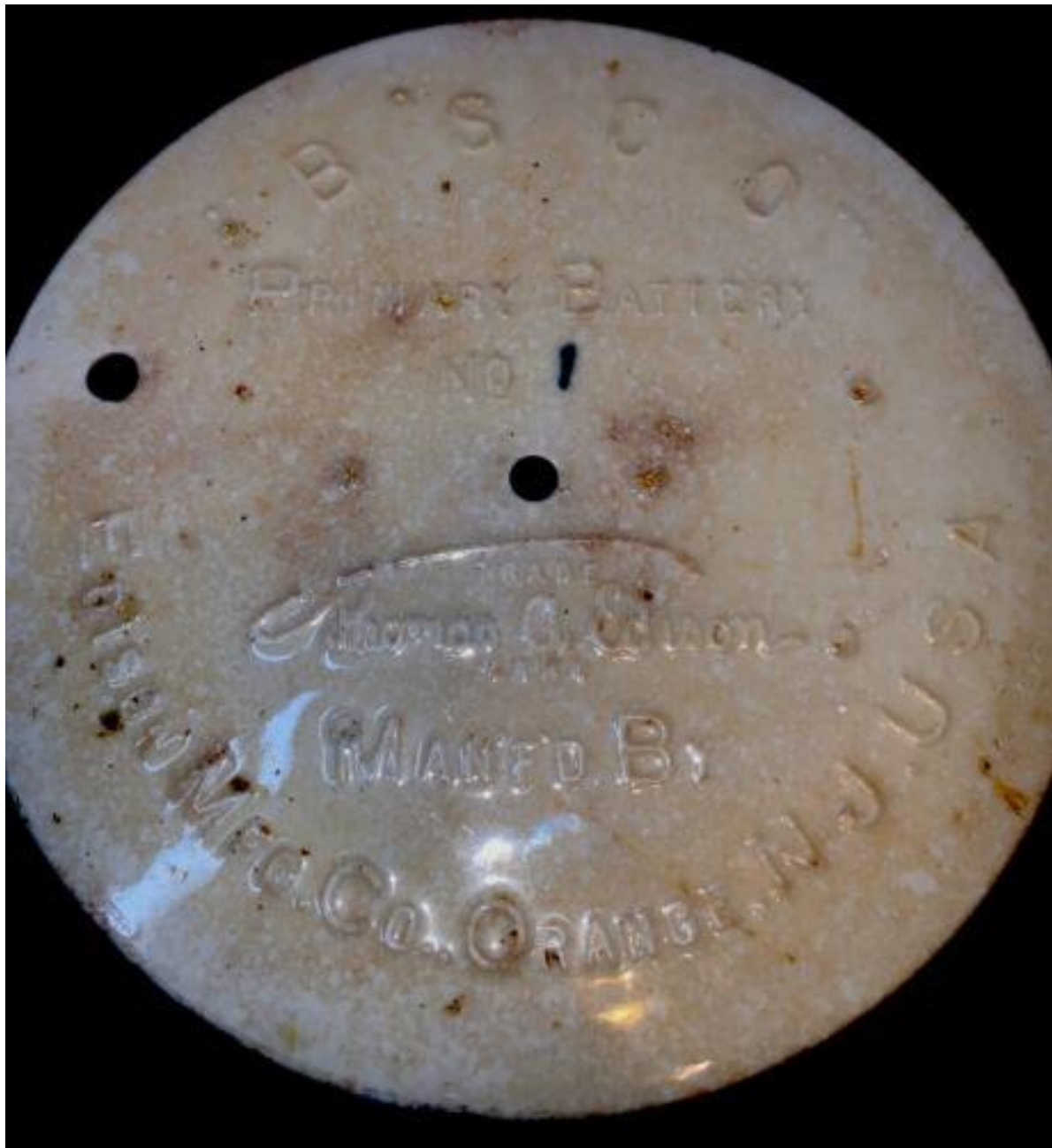
36.12 ↑ is an Edison Lid of Porcelain. It is 7" in diameter and embossed as follows: (Arc) ** B S C O ** / Primary Battery / No 1 / (Script) Thomas A. Edison / Manf'd By / (arc) Edison Mfg. Co., Oranbge, N.J. U.S.A.
