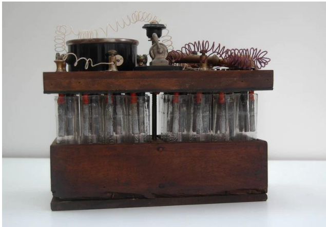
← 7.13 is a battery from a shock machine by Charles Chardin of France. Likely earlier than the porcelain ones shown above.
