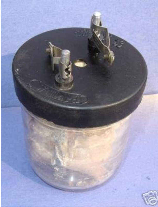
← 13.8 is a rectifier cell from Willard.
