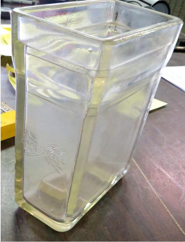
← 46.12 is Gamewell battery Jar embossed on opposing ends, with the Gamewell logo. It is 6.75" tall, while the sides flare. The base is 2.375" x 4.75", while the top is 2.875" x 5.375". It is straw colored with a formed lip. Courtesy of Tommy Bolack
